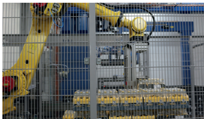
Behind the grating: Even the robotic palletiser can't function without (compressed) air.
